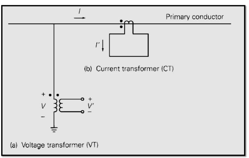
The current transformer has two jobs to do. Firstly, it steps down the current to such levels that it can be easily handled by the relay. Secondly, it isolates the relay circuit from the high voltage of the power system.
